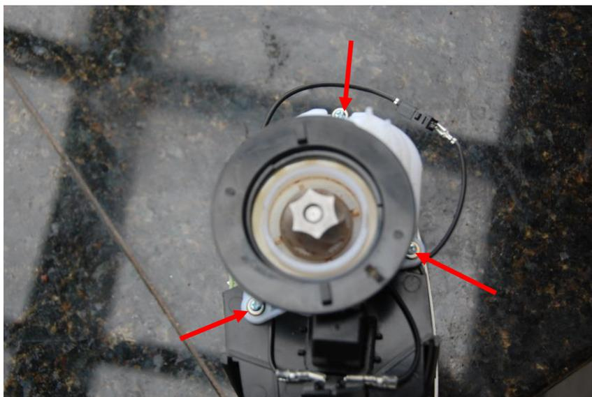
Then the two Phillips screws securing the power board are accessible. Unplug the wires, remove the two screws, and replace the board.
