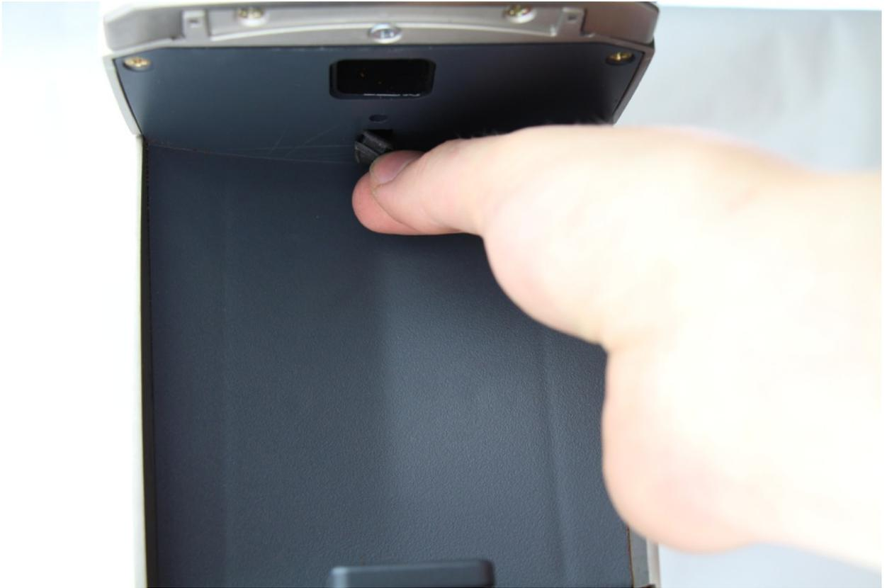
Pulling the 2.5mm screw towards the front of the grinder makes the grind **coarser**.
