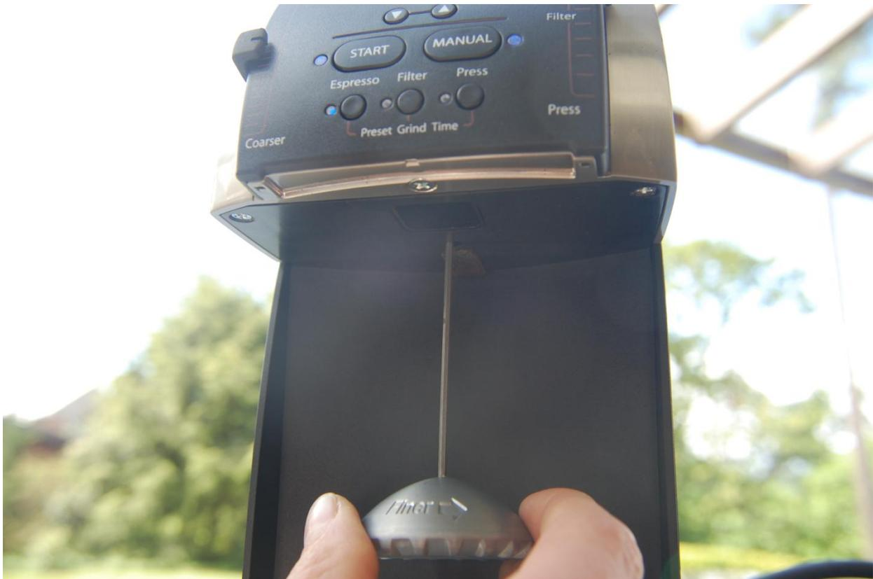
Slowly rotate the tool finer until you begin to hear the motor labor and change pitch. The burrs are beginning to touch at this point.
