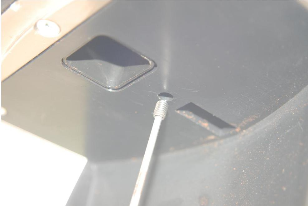
Loosen the 2.5MM Allen screw found in the rectangle slot. Again, **Please note that all calibration efforts need to be performed while the grinder is placed on the counter in the upright position.** Moving the screw towards the front of the grinder (arrow pictured below) makes the grind coarser. Then tighten the 2.5mm screw.
