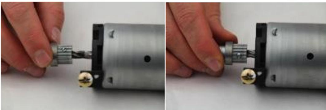
9. Tighten the set screw as much as possible. **Apply direct pressure while tightening to avoid slipping or injury by a blunt object.**
