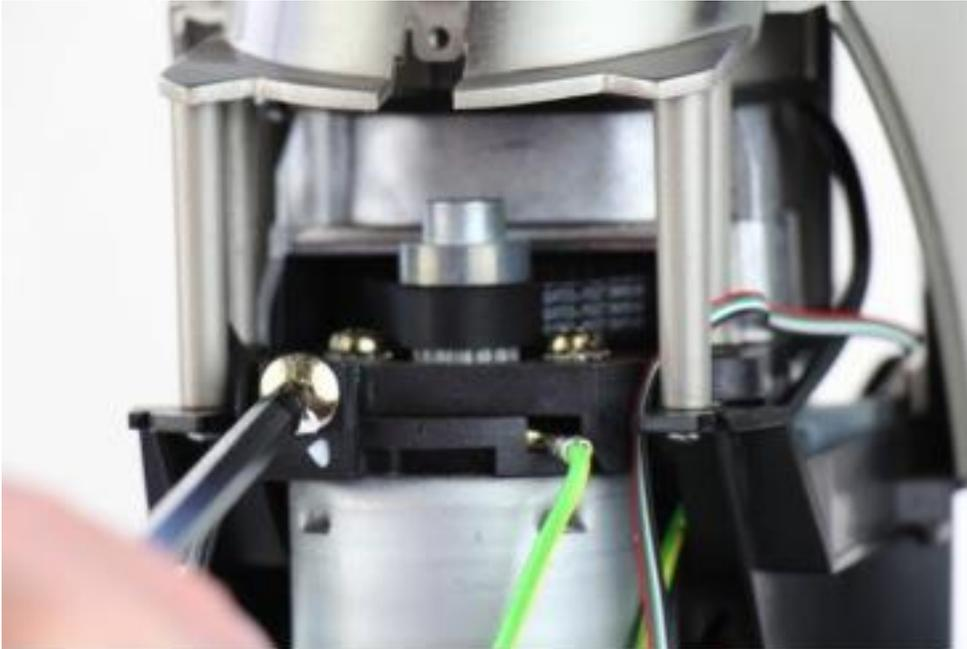
3. Loosen the motor tension screw, but do not remove it from the tension mount.
