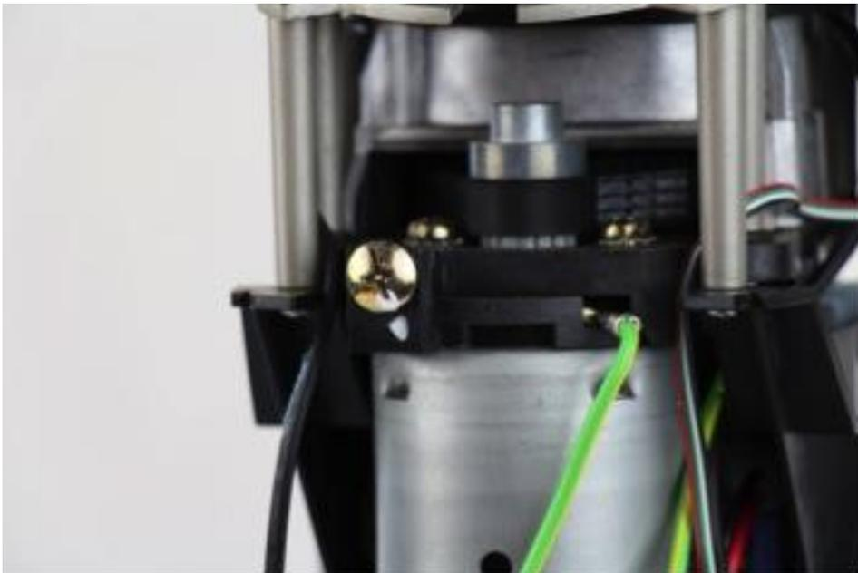
2. Rotate the screw exactly 1080 degrees (three full rotations) counterclockwise when loosening.
