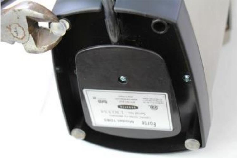
6. Remove the Philips self-tapping screws from beneath the rear two feet.
