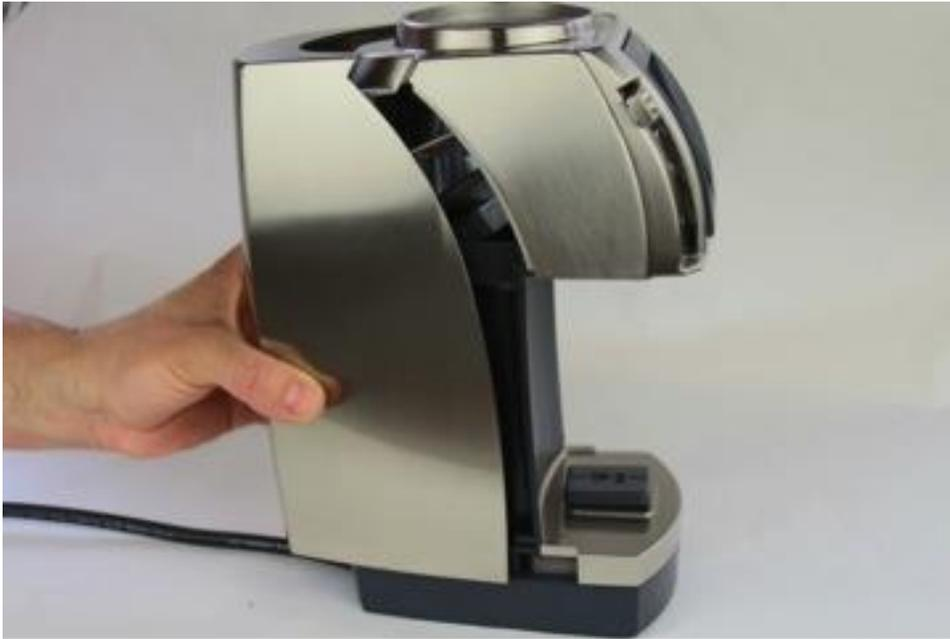
**With the casing removed, reinstall the hopper and plug in the grinder. Press TIME, M, then START. The motor should power on. If the motor powers on and is spinning, but the belt/pulley does not spin, then your pulley set screw needs to be reset. The motor must be removed to reset the set screw.**
